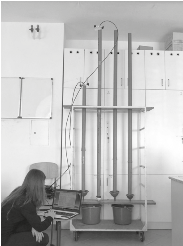
FIG. 9 - Laboratory investigation of clogging zone samples.
