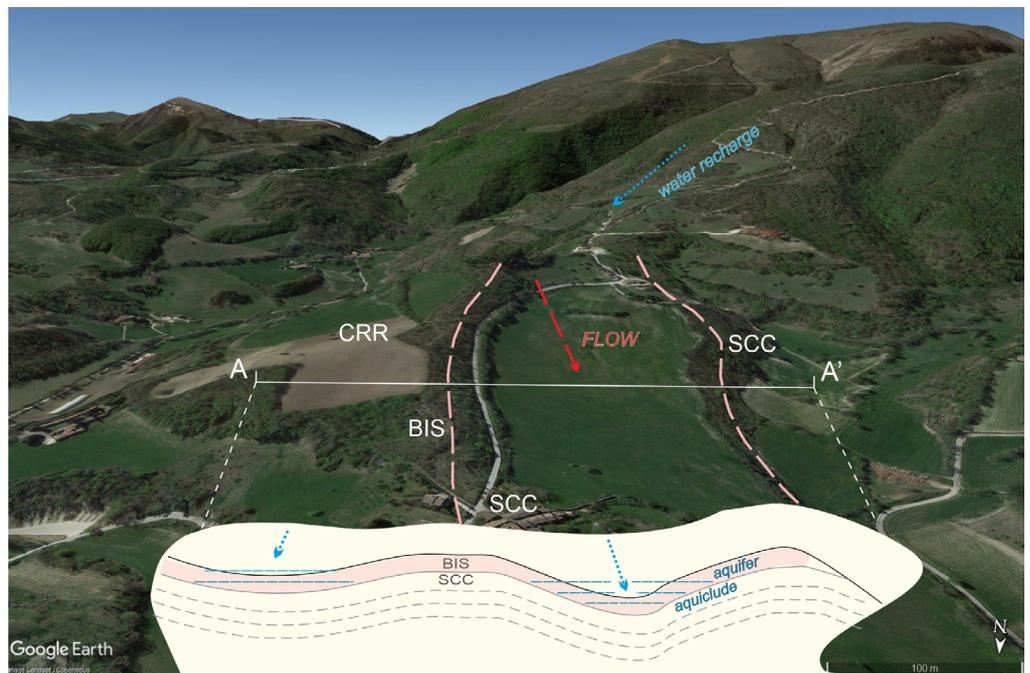
Figure 20 - Interpretative 3-D sketch of the hydrogeological structures that favour the accumulation and occasional overflow of water triggering flow landslides. CRR (Marne con Cerrognna), BIS (Bisciario) and SCC (Scaglia cinerea) represent the bedrock formations; A-A' schematic cross section (base image from Google Earth, 2024).
