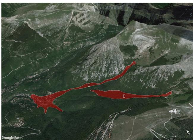
Figure 5 - 3D view of the sketch map of the last Varluscio Landslide Event (in red) (Google Earth aerial view).
