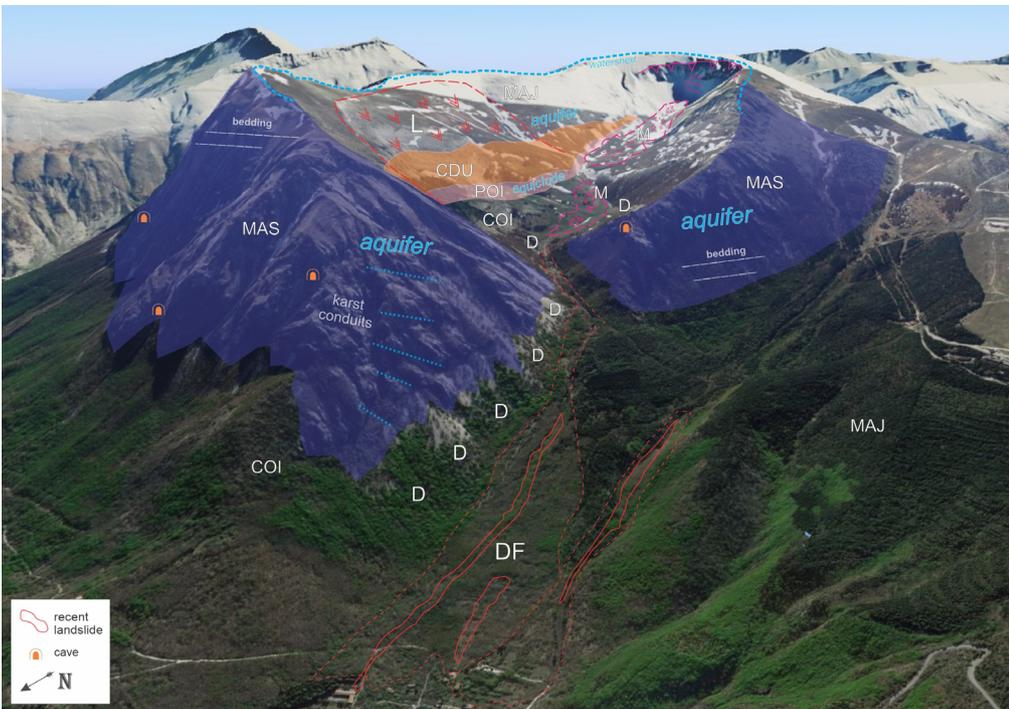
Figure 18 - Geological and geomorphological sketch interpreting the dynamics of processes in the VU area (Monte Bove relief). MAS-Calcare massiccio, COI-Corniola, POD-Marne a Posidonia, CDU-Calcarei Diasprini U.M., MAJ-Maiolica, M- relict glacial deposits, L-gravitational movements, D-coarse Debris and blocks, DF-debris flow area, in continuous red line the recent ones (base image from Google Earth, 2024).
