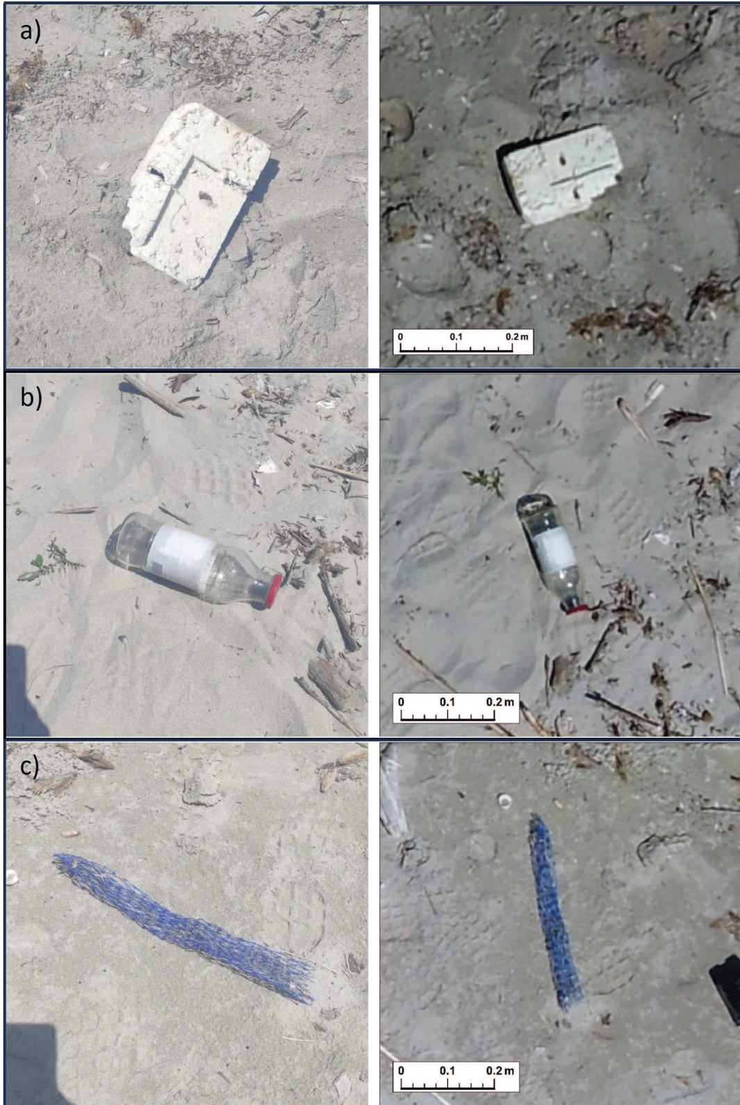
FIG. 4 - Examples of litter items identified during the in-situ survey and their corresponding identified by the manual image screening in GIS environment: a) polystyrene pieces (J82), b) drink glass bottle (J200), and c) net for mussel/fishing activities (J45).
