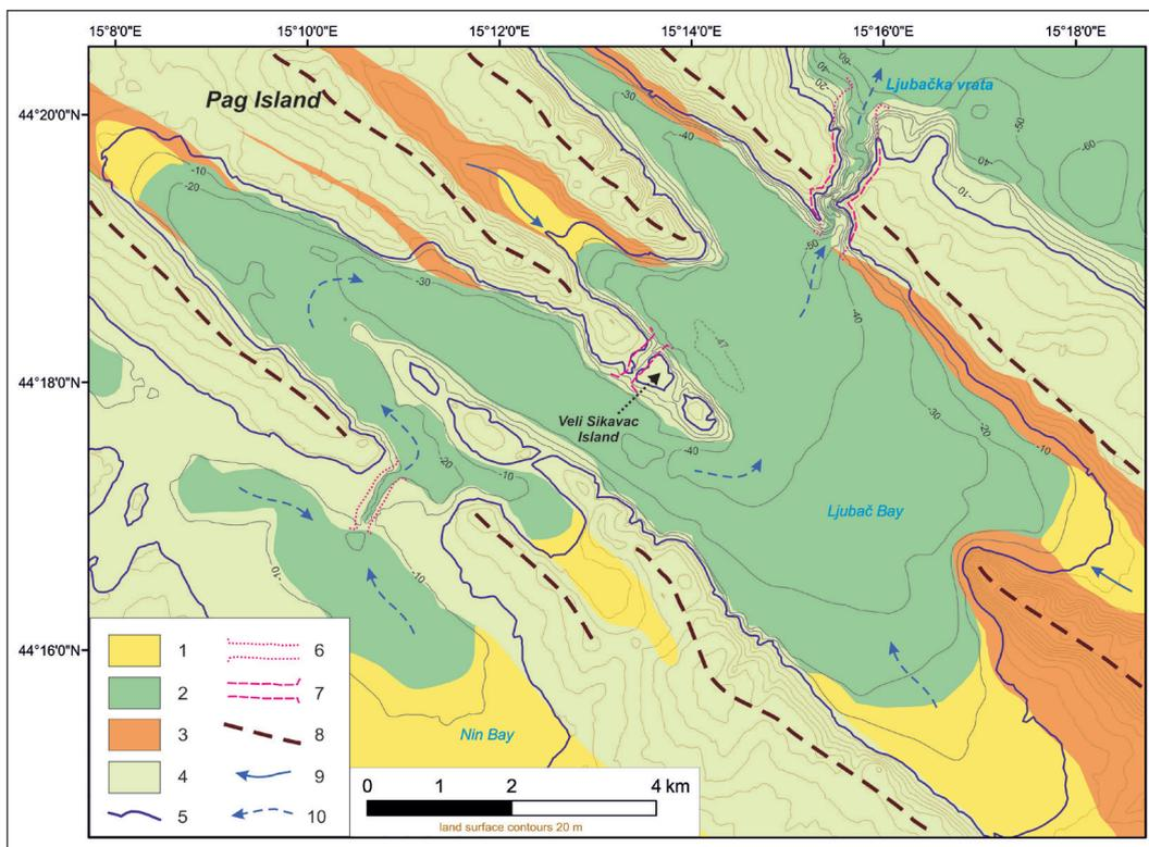
FIG. 5 - Geomorphological sketch map of subaerial and submerged landforms of the Ljubač Bay: 1) alluvial-proluvial sediments; 2) marine sediments; 3) flysch rocks; 4) carbonate rocks; 5) recent coastline; 6) submerged canyon; 7) partially submerged canyon; 8) main ridges; 9) surface flow; 10) presumed flow during lowstanding sea-level.
