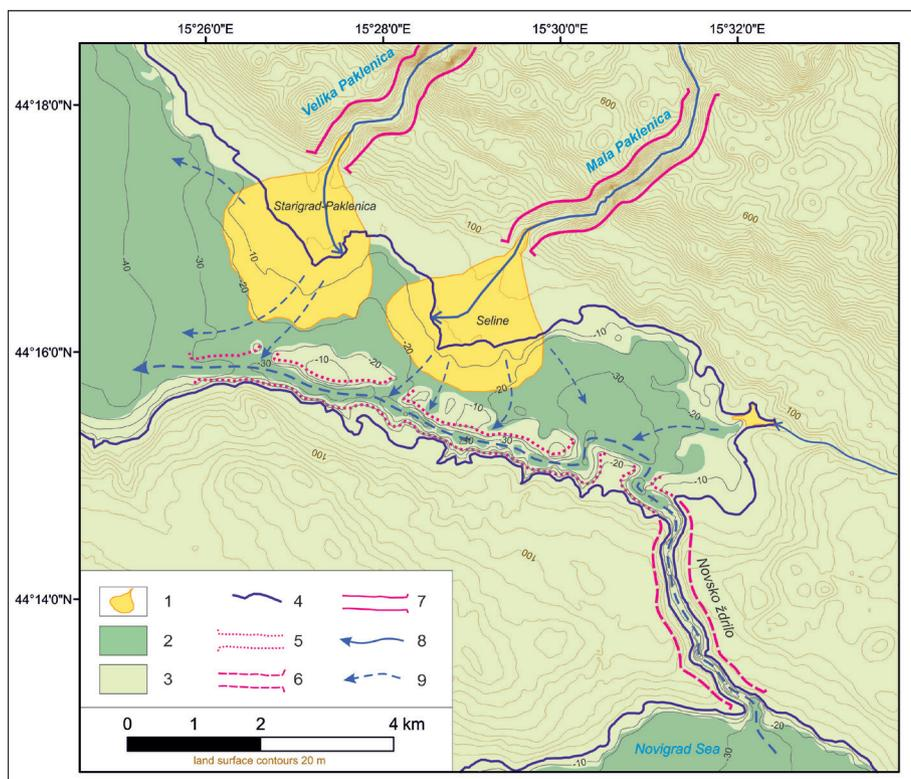
FIG. 4 - Geomorphological sketch map of subaerial and submerged landforms of the Velebit Channel and the Novigrad Sea: 1) alluvial fan; 2) marine sediments; 3) carbonate bedrock; 4) recent coastline; 5) submerged canyon; 6) partially submerged canyon; 7) canyon; 8) surface flow; 9) presumed paleoriver flow during lowstanding sea-level.
