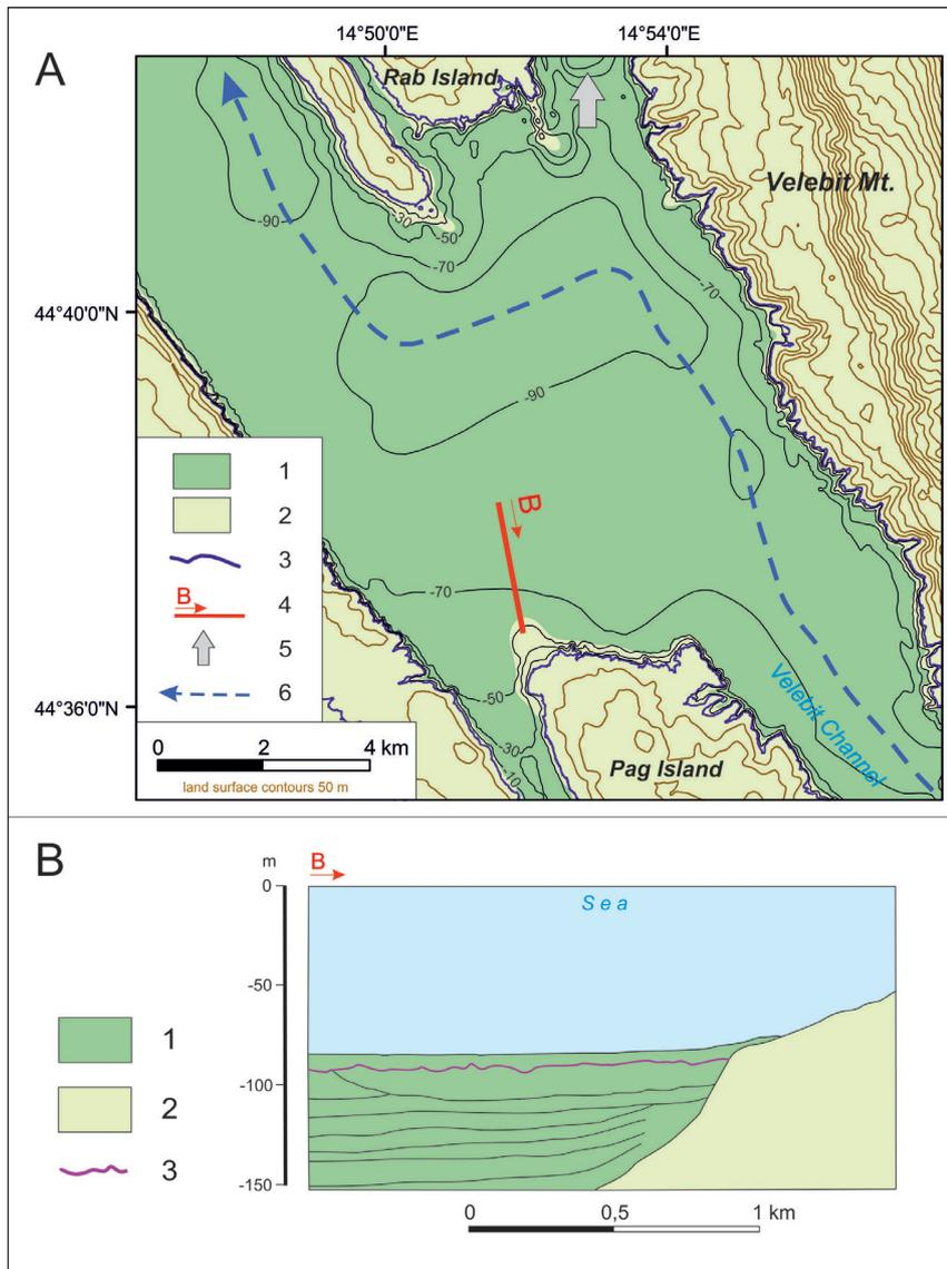
FIG. 8 - A) Geomorphological map of subaerial and submerged of NW part of the Velebit Channel: 1) marine sediments; 2) carbonate rocks; 3) recent coastline; 4) trace of sub-bottom cross-section; 5) location of shallows; 6) paleo riverbed; B) geological cross-section (after Benac & alii, 1995): 1) marine sediments; 2) carbonate rocks; 3) erosional disconformity.
