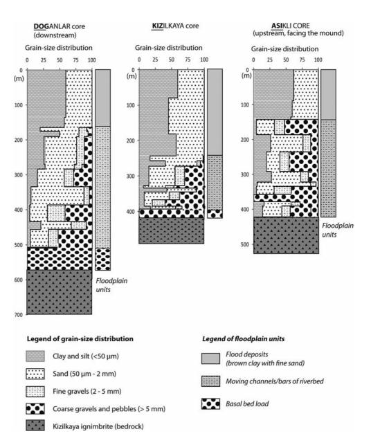
Aşıklı mound downstream to the Doğanlar village facing Kızılkaya village. The 64 mm diameter cores were extracted using a rotary and hydraulic Craelius XC-SH truck mounted drill. Cores were sub-sampled at the coring spots, with intervals based on the facies and estimated grain size of the stratigraphic units identified during the coring process. Samples were sent to Laboratoire de Géographie Physique (LGP) in Meudon (France) for analyses.
