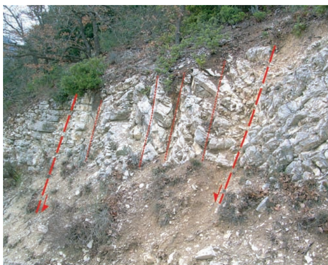
FIG. 9 - Borgiano area: E-W discontinuities forming a geological mini-graben in the middle portion of the slope.
