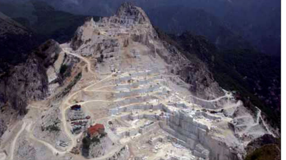
Gioia Quarry (Colonnata Basin) The marble extraction spreads over a number of fronts that have affected Cima Gioia. Access roads run on dump deposits and reach several active quarry fronts (May 30, 2003).
