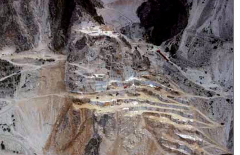
Overview of the quarry area near Lorenzo Active and inactive quarry areas, access roads, and dump deposits with different classes of texture and degrees of weathering developed all over the area. Dumping channel tracks arise from the quarry yards. Debris flow channels and lobes are observed in the upper right of the photograph (May 20, 2003).
