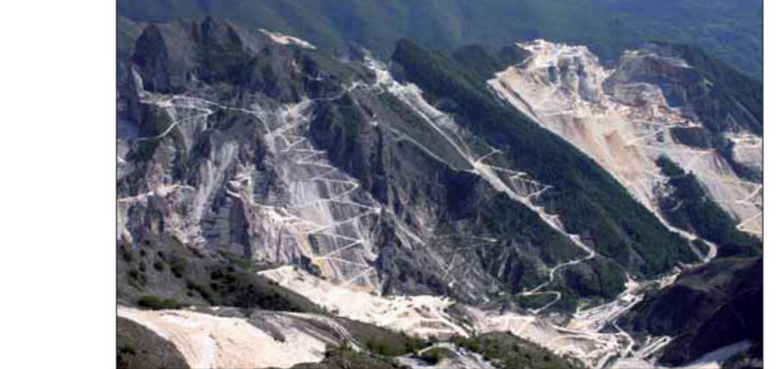
Overview of the Ravavione area in the Torano Basin (from Campocecina) The quarries of Cima Caravignolo (on the left) and ancient and weathered quarry dumps (gray in the picture). Active quarry dumps (light gray in the picture) on the top of the stoneblock run. Weathered quarry dumps with vertical benches are used for the secondary sculpture, from the ancient quarries of the Ravavione Basin (May 18, 2006).
