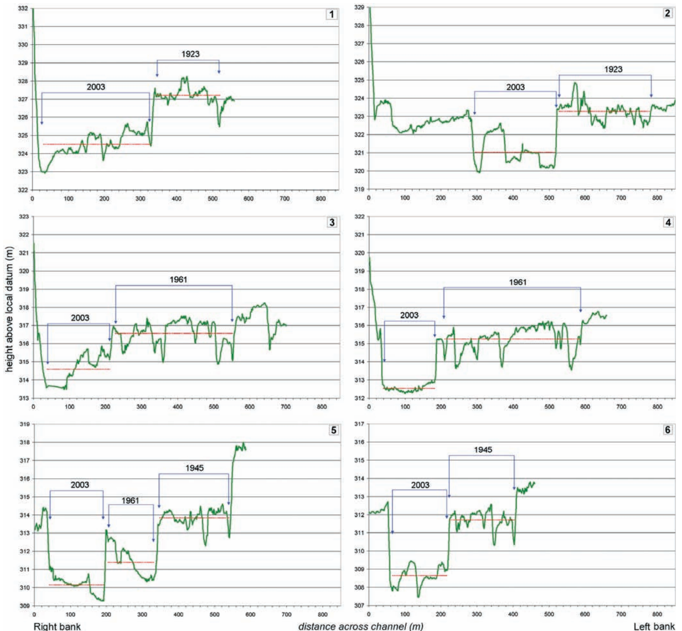
FIG. 8 - The six cross-sections, drawn out from the 2003-DTM, are numbered 1 to 6 from upstream to downstream. The positions of the present channel (2003) and of the remaining portions of the older ones (occupied until 1923, 1945 and 1961) are given. The red lines show the mean level of the river bed in different years.
