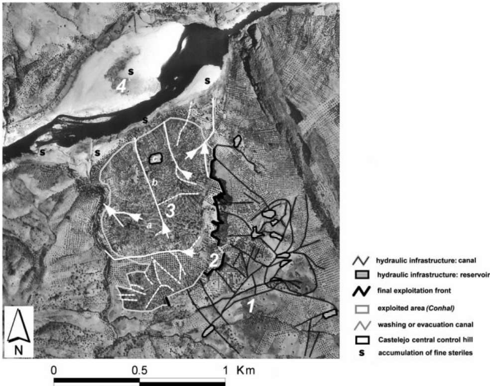
FIG. 4 - Different sectors of the historical gold exploitation [Aerial photograph dating from 1958, before construction of the Fratel dam (1973)]. Legend: 1. Water supply zone; 2. Final exploitation front; 3. Exploited area - a. Boulder piles ( muria ); b. Washing and evacuation canals; c. Castelejo control hill; 4. Accumulation of evacuated fine steriles (photo provided by the Fundação Cidade de Ammaia, Marvão, Portugal, original scale: 1:20,000, series 57AM29).
