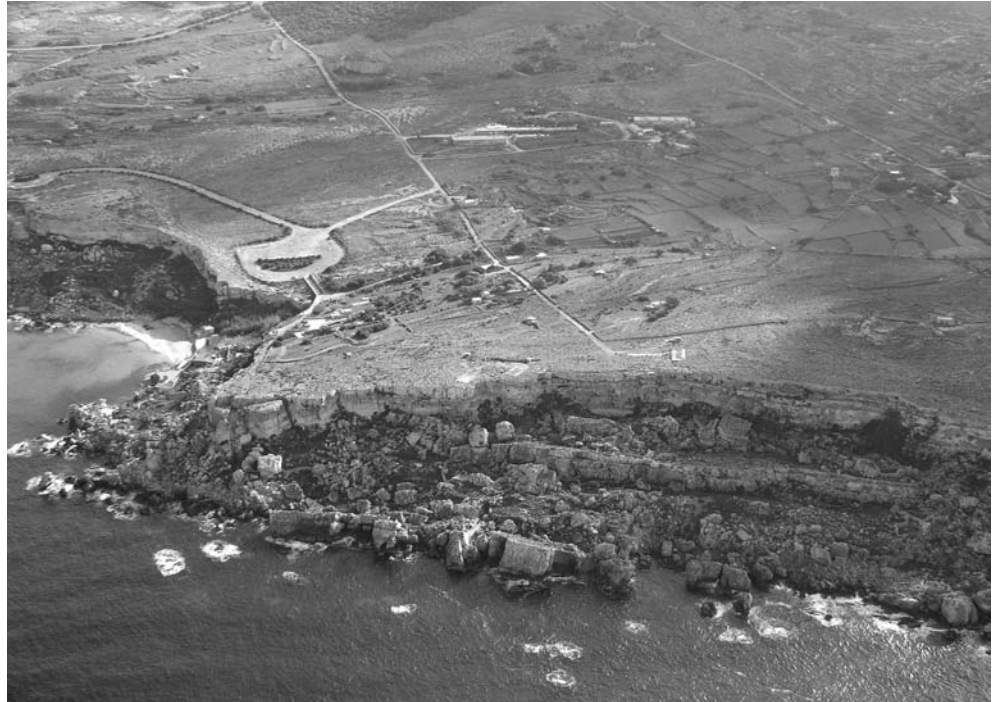
FIG. 3 - Lateral spreading along the north-west coast of Malta develops due to the superimposition of Upper Coralline Limestone which overlies the Blue Clay. Limestone blocks extend over the clay material and even act as buttressing to the shoreline (courtesy of Patrick Bonnici).
