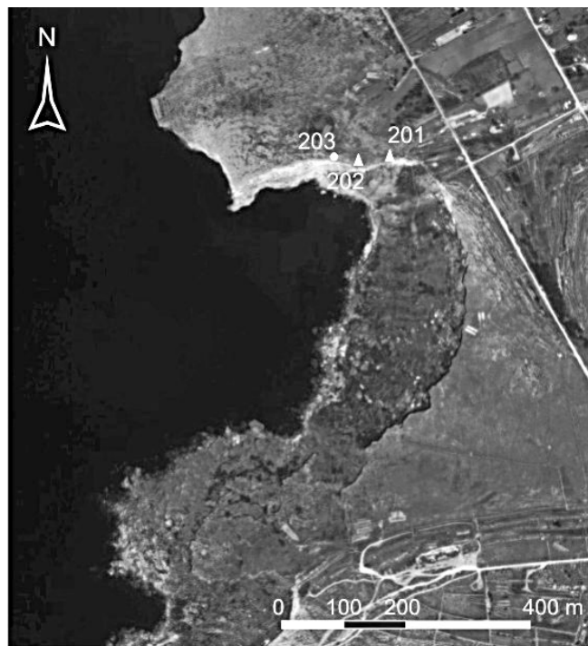
FIG. 6 - Satellite image of Rdum id-Delli: benchmarks that recorded significant planar displacements are indicated with a triangle symbol, those which have moved during the wet period are indicated with a circle symbol.
