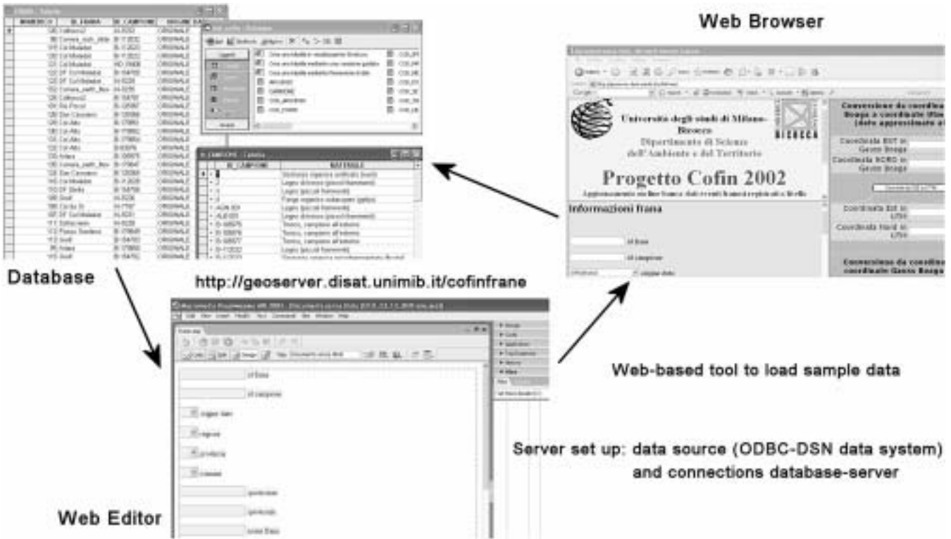
FIG. 2 - Server-client architecture used in the uploading of the data into the data base.
