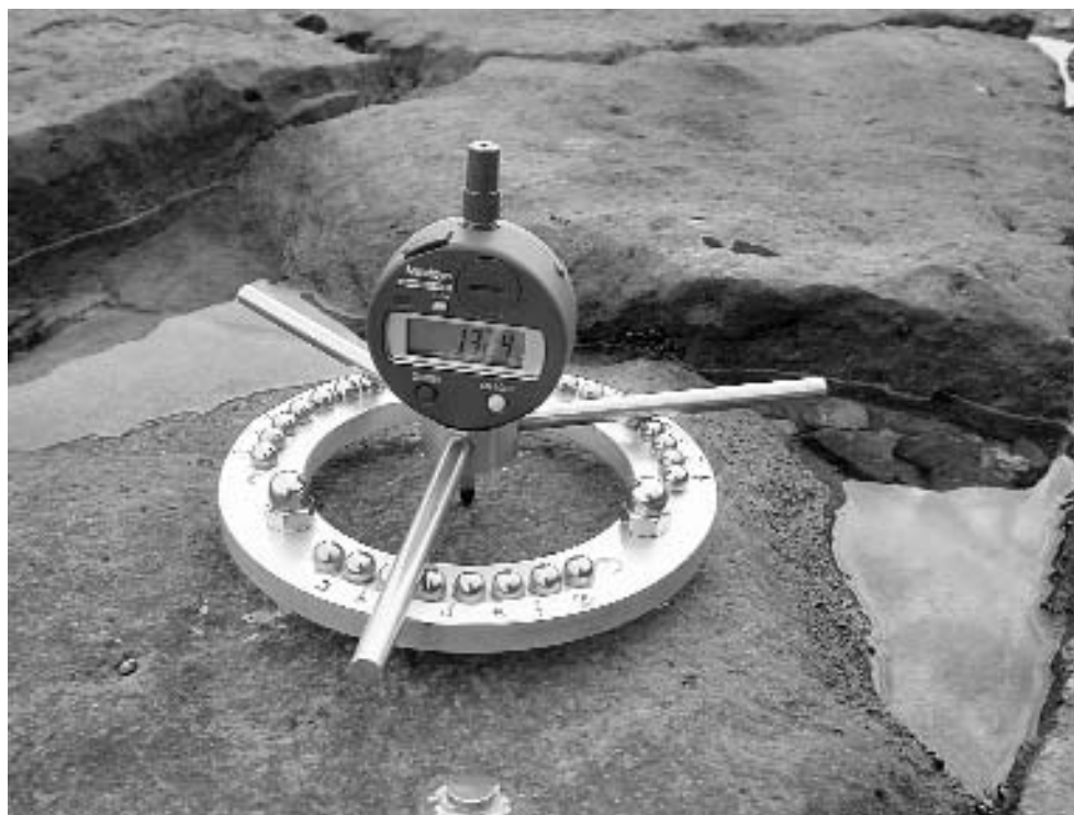
FIG. 2 - The traversing micro-erosion meter (t-MEM) used by the authors.
