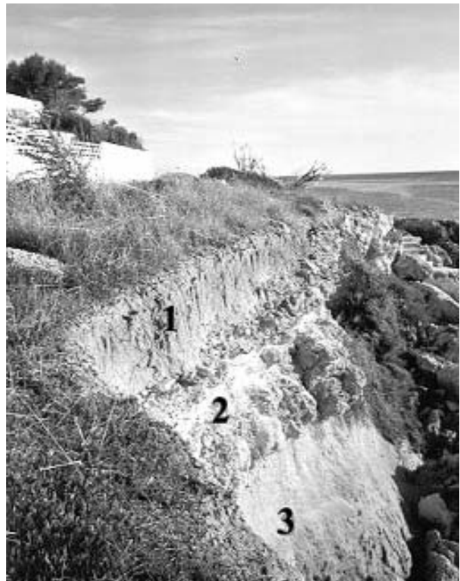
FIG. 5 - Cliff in Battaglia zone near Taranto; it is possible to observe a detaching niche of a recent collapse and the local stratigraphic sequence: 1) soil about 90 cm thick covered by gariga ; 2) Raised beach (Upper Pleistocene) (thickness: 1,3 m); 3) Argille subappennine (Late and Middle Pleistocene) (thickness between 6-8 m).
