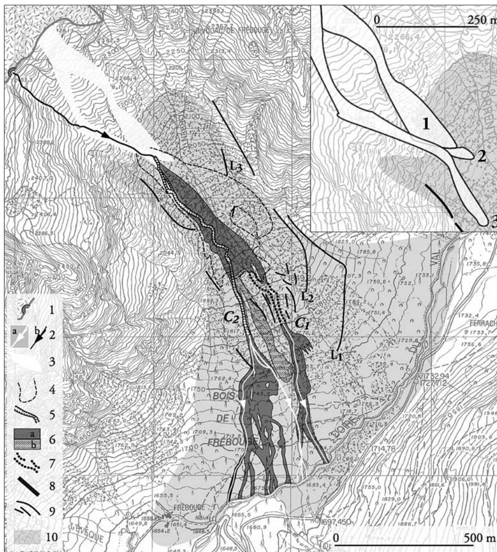
FIG. 2 - Frébouge debris flow deposits map (from terrestrial photographs). 1: Glacier de Frébouge front and portal; 2: proglacial torrent (a: downstream section; b: up stream section); 3: 17 July ice avalanche deposits; 4: limit of September 2002 ice avalanche deposit; 5: new incised channel; 6: 17 July debris flow deposit (a: coarse deposit; b: detrital veneer); 7: debris flow levees; 8: 20 July debris flow deposit; 9: LIA moraines (L 1 , L 2 , L 3 generations); 10: Frébouge polygenic fan area. Box: 17 July ice avalanche deposits, in order of occurrence. [topographical map 1:10000; contours: 10 m. Archivi topocartografici della Regione Autonoma Valle d'Aosta Permit n. 52 (18.08.1999)].
