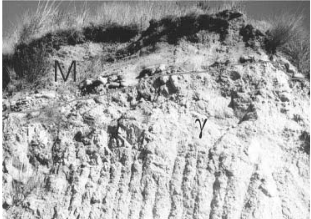
FIG. 4 - Transgressive miocenic conglomerates and sands on highly fractured and mildly altered granitoids ( \gamma ) - values of rebound to the Schmitt hammer up to 20-25.
