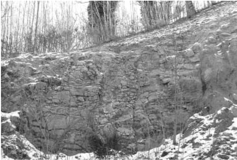
FIG. 7 - Immature Saprolite (Class IV-V-IAEG) in outcrop. The corestones to the Schmidt hammer gives values up to 20-25.
