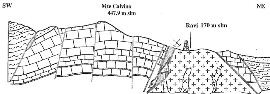
FIG. 3 - Geological cross section directed NE-SW and passing through the Mt. Calvo area.
