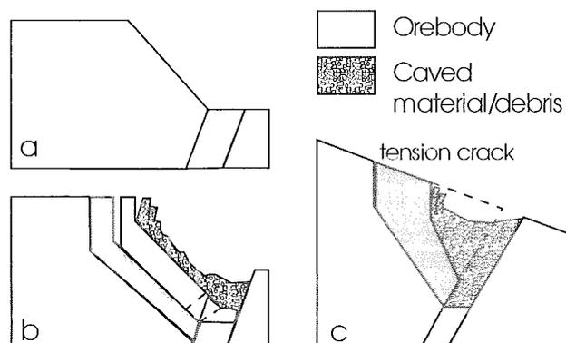
FIG. 7 - a) HOEK's model (1974) and b) BROWN & FERGUSON's model (1979) for progressive hangingwall caving along sloping ground.
