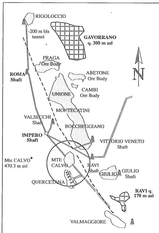
FIG. 2 - Sketch showing the location of main ore bodies (not in scale), adopted names and more important drifts and shafts.
