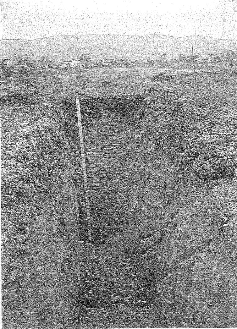
FIG. 4 - Close-packed horizons classified as pedal dense subsurface horizons are not brittle and the bleached streaks are not coarser than the matrix. They show different types of prismatic or angular blocky structure.
