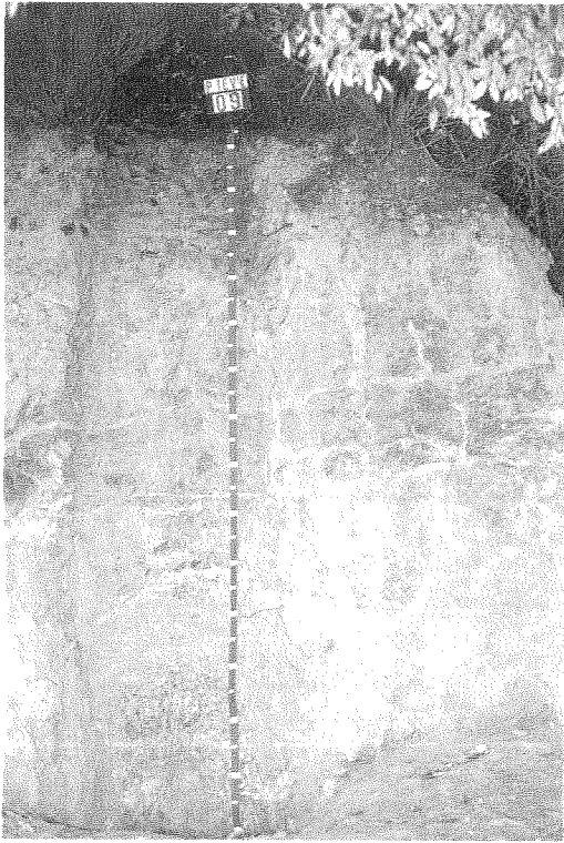
FIG. 1 - Some soils of the Montagnola Senese area have a subsurface close-packed horizon matching the diagnostic criteria of a true fragipan.
