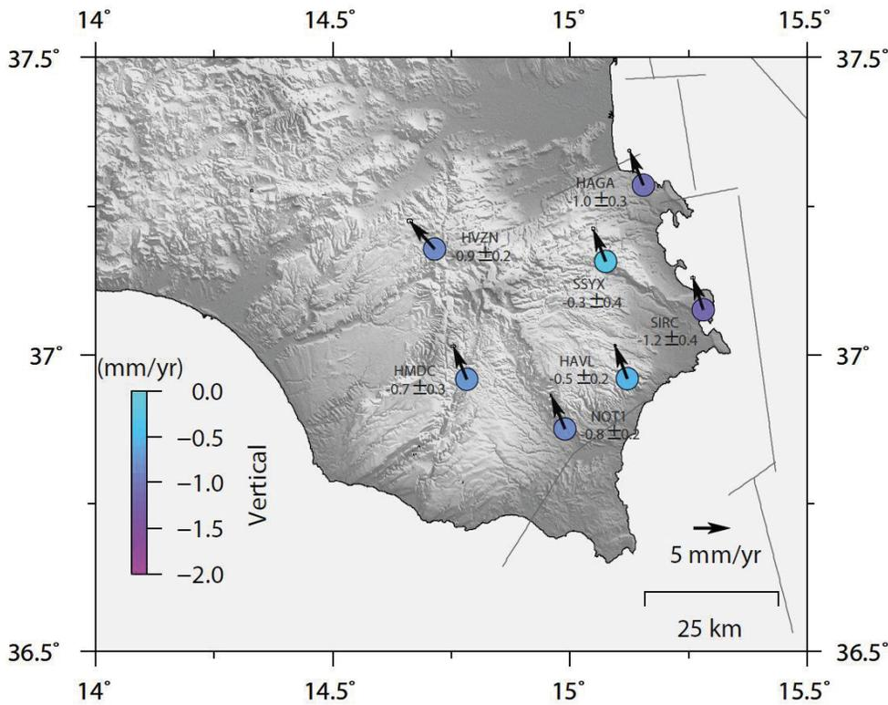
FIG. 5 - The CGPS stations belonging to the INGV-GNSS network, located in the surroundings of the studied area. Arrows are the horizontal motion at the individual stations, while in colour are the vertical velocities with related values and uncertainties (see color palette for scale).
