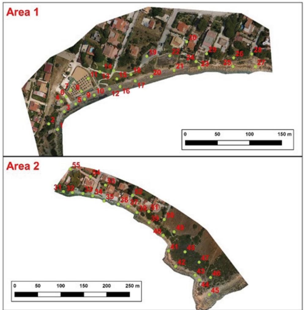
FIG. 4 - Position of the Ground Control Points (GCPs) measured in the investigated area.
