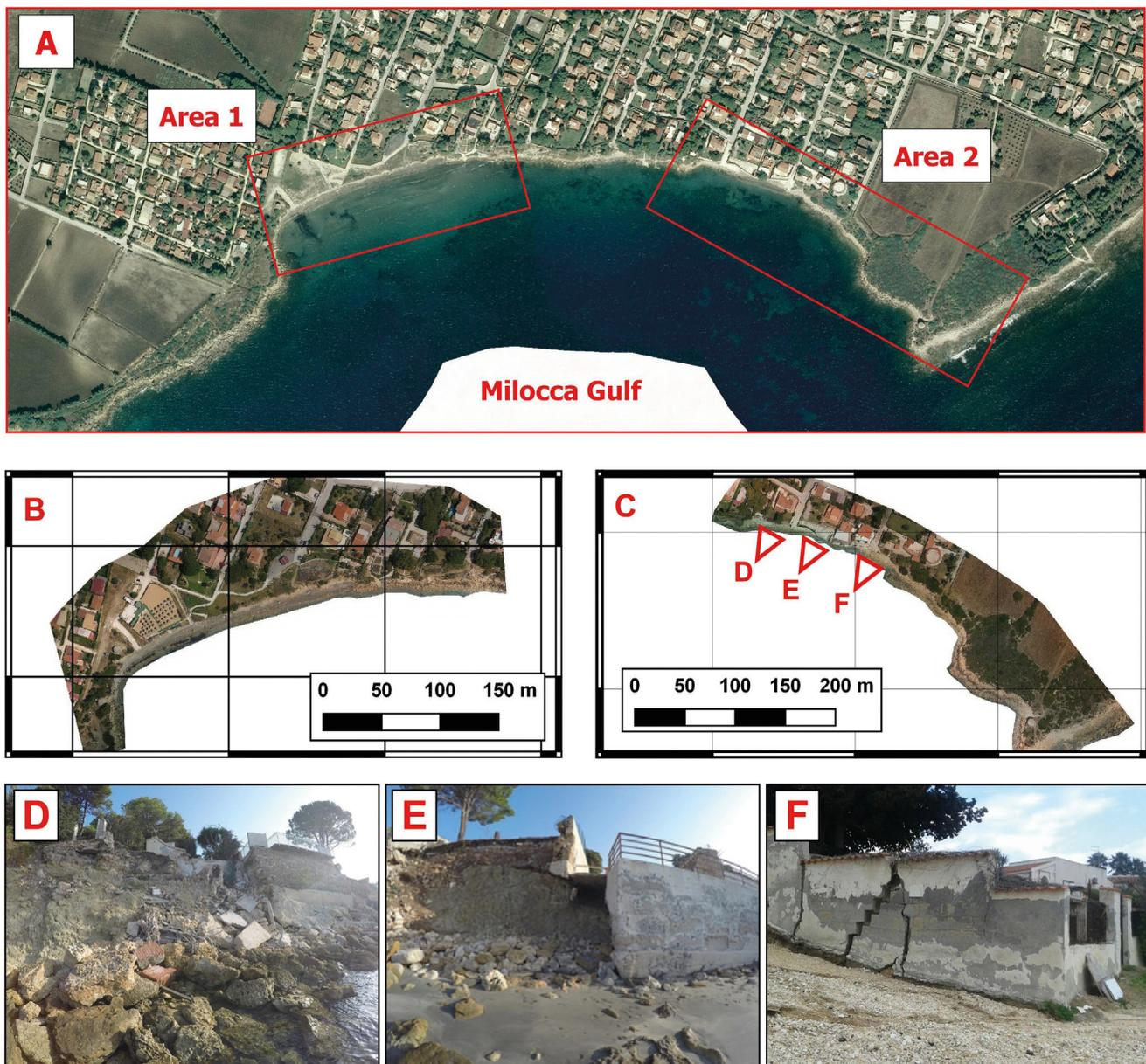
FIG. 2 - A) UAV survey area; B) Area 1; C) Area 2; D) Collapsed houses along the shoreline; E and F) Details of the collapses caused by coastal erosion.
