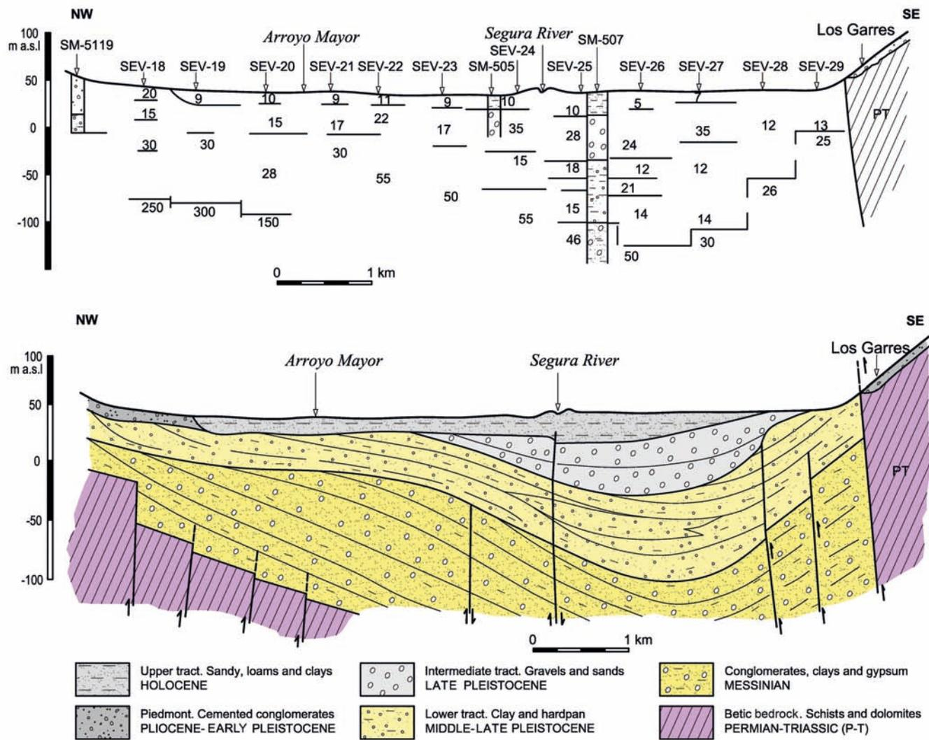
FIG. 7 - Geological and tectonic cross-section I-I' (see location in Fig. 1) of the Vega Media of the Segura River (Rodríguez-Estrella & *alii*, 1999). Source: geophysical and mechanical boreholes data.
