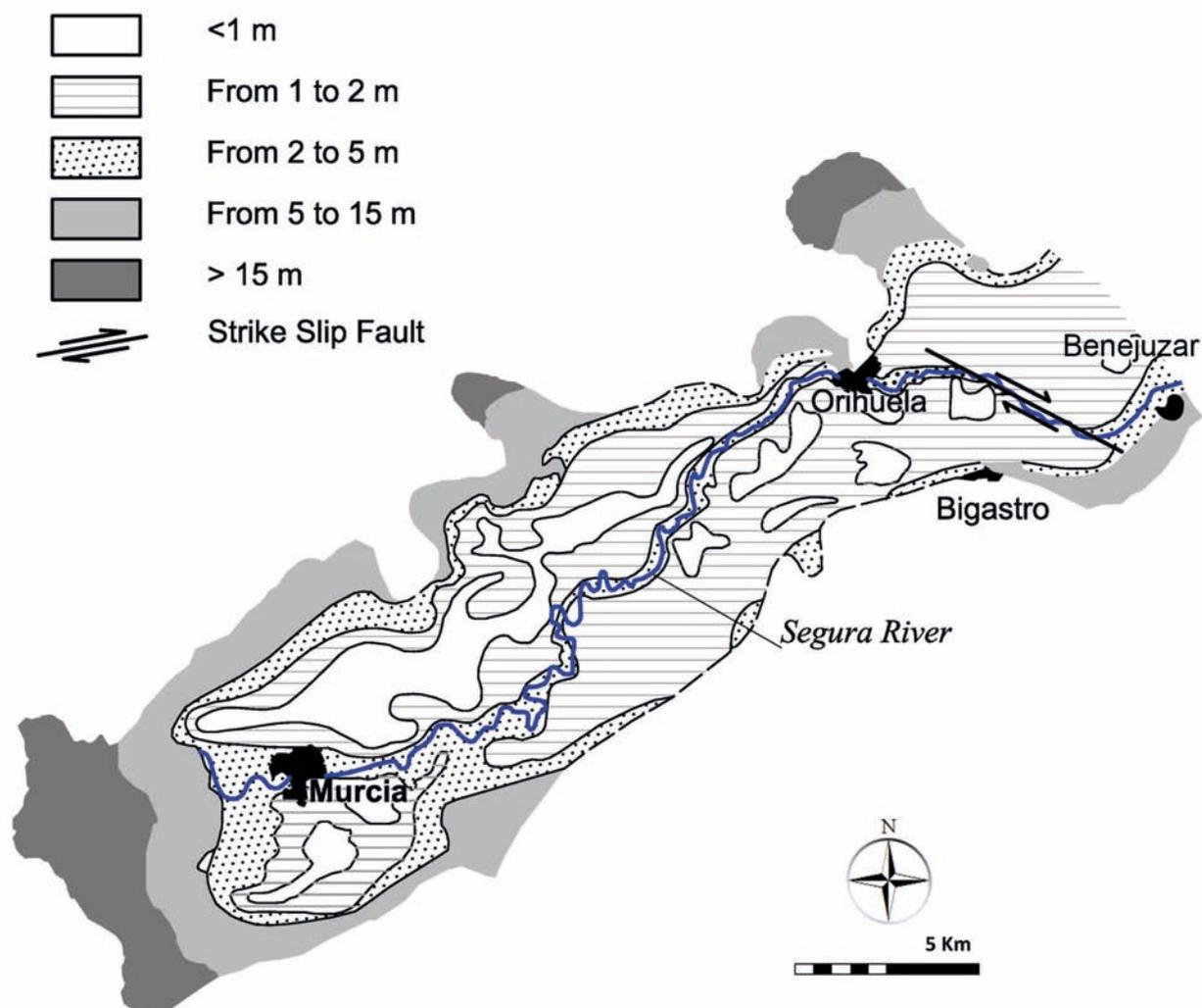
FIG. 3 - Isodepths map of groundwater associated with silts, according to data collected in 1972-73 (Rodríguez-Estrella, 1983).
