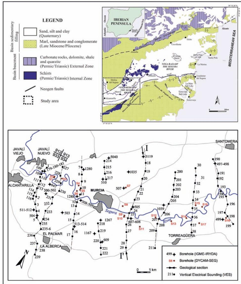
FIG. 1 - Geological setting of the Vega Baja and Media of the Segura River Basin (based on Montecat, 1977) (upper part); location of the mechanical surveys and geophysical VES carried out by the IGME-IRYDA in 1975 (Rodríguez-Estrella & *alii*, 1999), and of the boreholes installed in the project DYCAM-SEG (2010-2015) (lower part).
