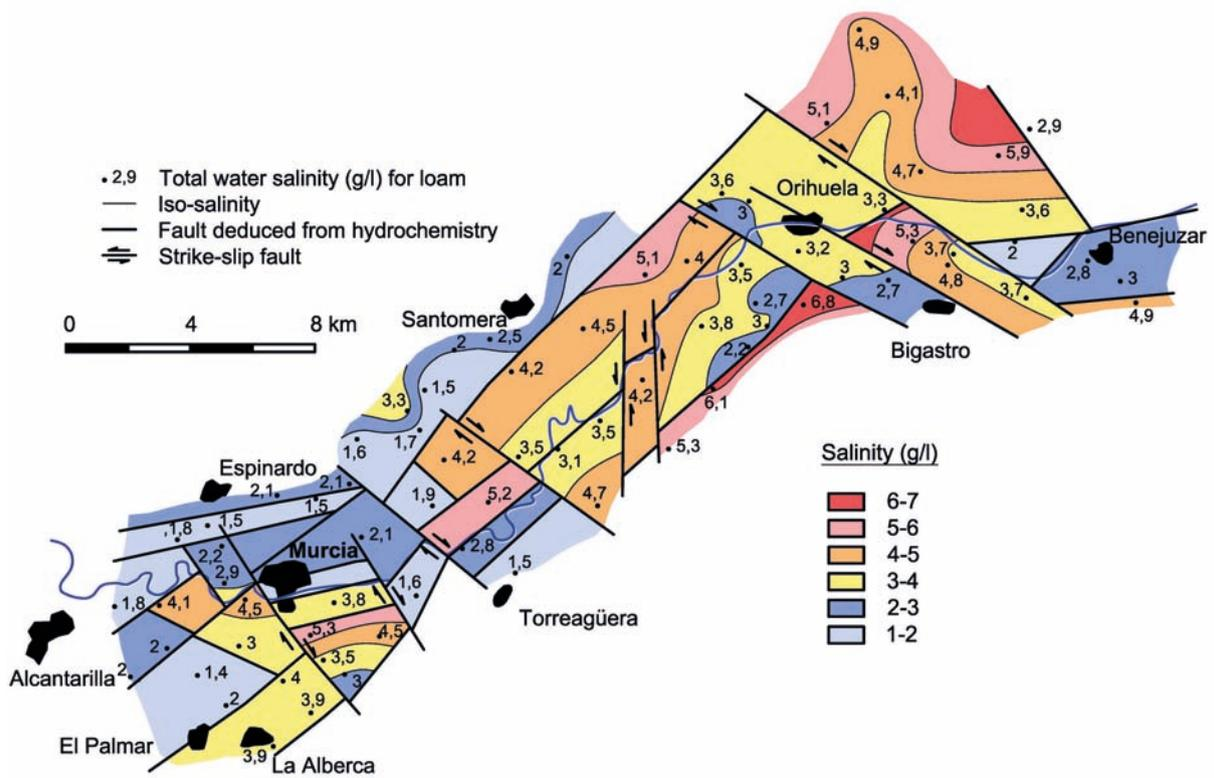
FIG. 4 - Faults deduced from the values of total salinity of the groundwater associated with silts.
