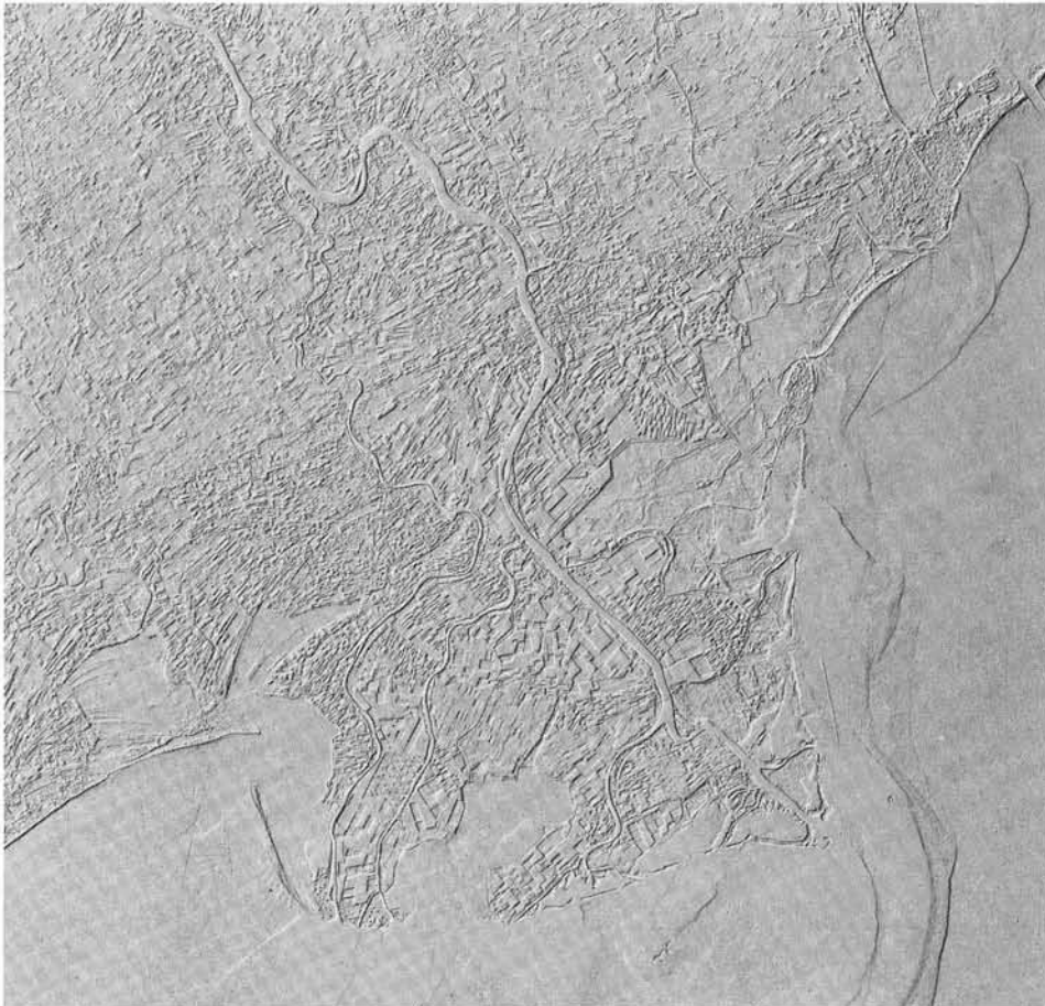
FIG. 9 - Pseudo-plastic presentation of the raster image: Accentuation of gray tone edges and line elements (Image processing by J. HENKEL, Munich).
