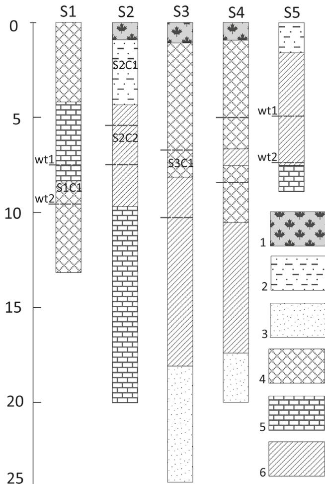
FIG. 5 - Borehole stratigraphies: 1. Organic soil; 2. Silty and clayey sands; 3. Marine sands; 4. Fractured shales with silty interlayers; 5. Shales and limestones; 6. Very fractured shales and limestones with silty interlayers. wt1-wt2: range between maximum and minimum water table values registered between 2003 and 2004. SC = Soil Sample (see Table 1 for further explanations).
