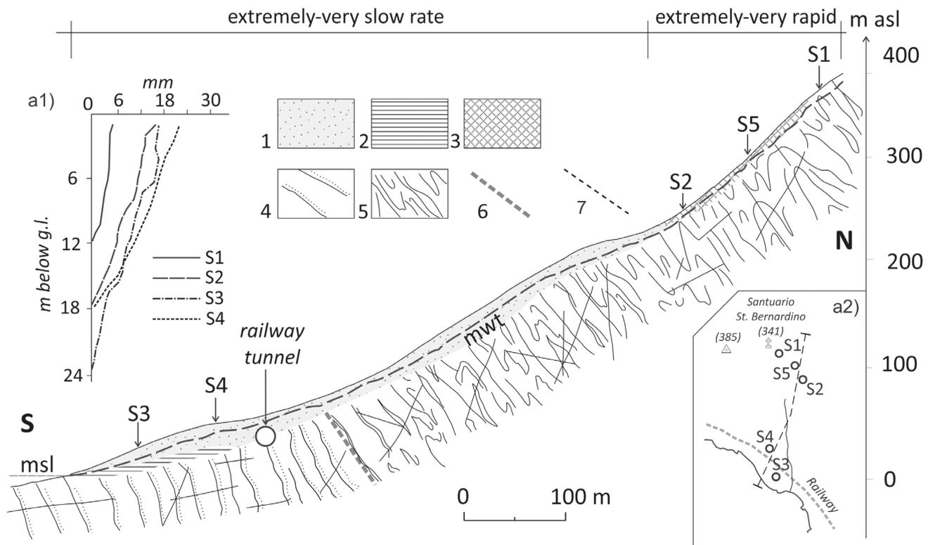
FIG. 4 - Geological cross section of S. Bernardino - Guvano landslide. 1. Medium/lower landslide body (silty and clayey sand); 2. Marine sands; 3. Upper landslide body (boulders and debris); 4. Sandstone (MAC); 5. Shales and limestone (ACC); 6. Fault; 7. Mean water table (mwt); a1: Inclinometer cumulative displacements profile during the 2003-2004 campaign time range; a2: Inset map showing borehole locations (S1-S5).
