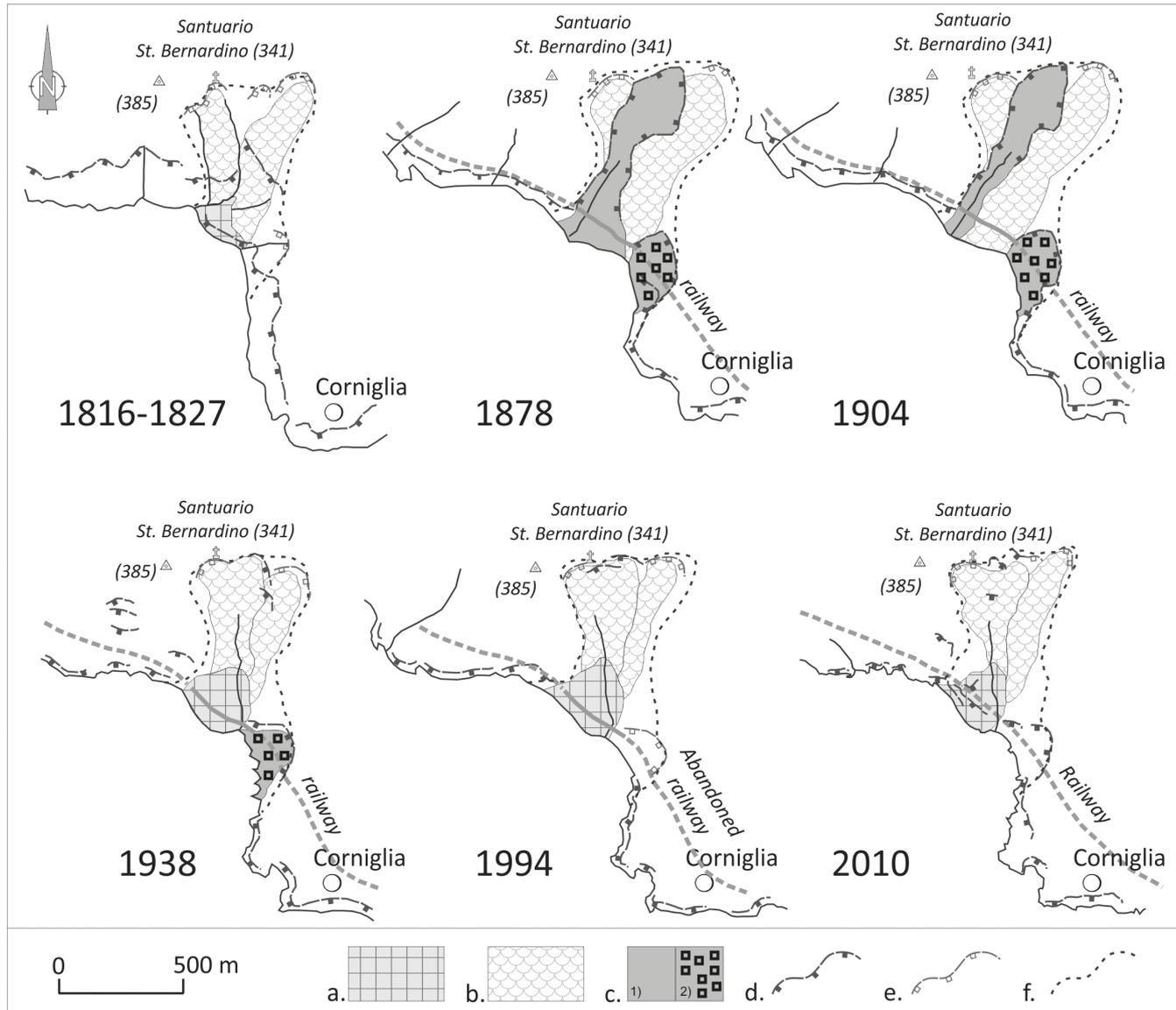
FIG. 6 - S. Bernardino - Guvano landslide evolution in the last two centuries: a. Talus flow; b. Complex landslide; c1. 1853 Landslide; c2. Rockfalls; d. Edge of active scarp; e. Edge of inactive scarp; f. Limit of ancient landslide.
