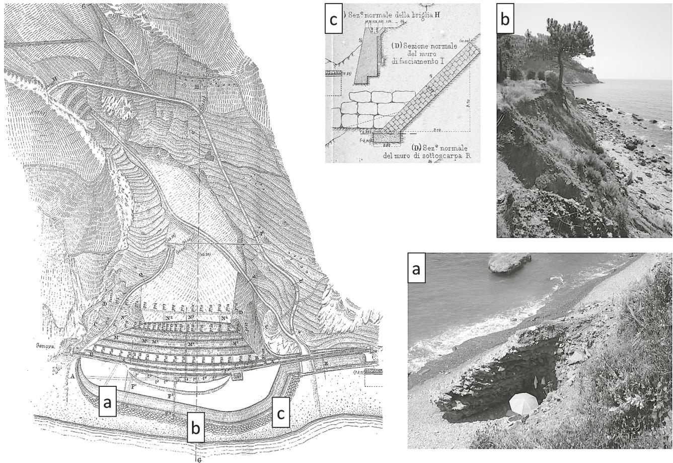
FIG. 2 - Interventions design to stabilize the S. Bernardino – Guvano landslide area realized by the “Ferrovie del Regno” Engineers (DIREZIONE TECNICA GOVERNATIVA, 1880): a) Ruins of the retaining wall (landslide toe); b) Active scarp due to sea wave erosion (landslide toe). c) retaining wall at the landslide toe.
