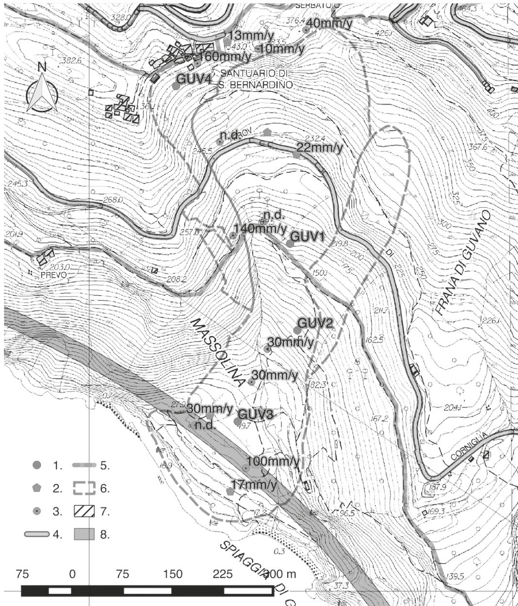
FIG. 8 - Slope dynamic sketch map: 1. GNSS sensors (2015-2016); 2. Inclinometers (2003-2004, after EPTACONSULT S.C.R.L., 2004); 3. Topographic landmarks (2003-2004, after EPTACONSULT S.C.R.L., 2004); 4. SP51 County Road; 5. SVA; 6. S. Bernardino-Guvano coastal landslide; 7. Urban areas; 8. Railway tunnel.
