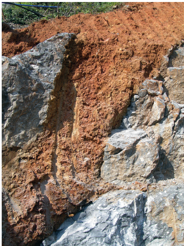
FIG. 9 - Deep weathering in fissures and cracks at the base of an terraced soil. Note the abrupt contact between the residual soil material and the reworked terraced infill. Trowel for scale.
