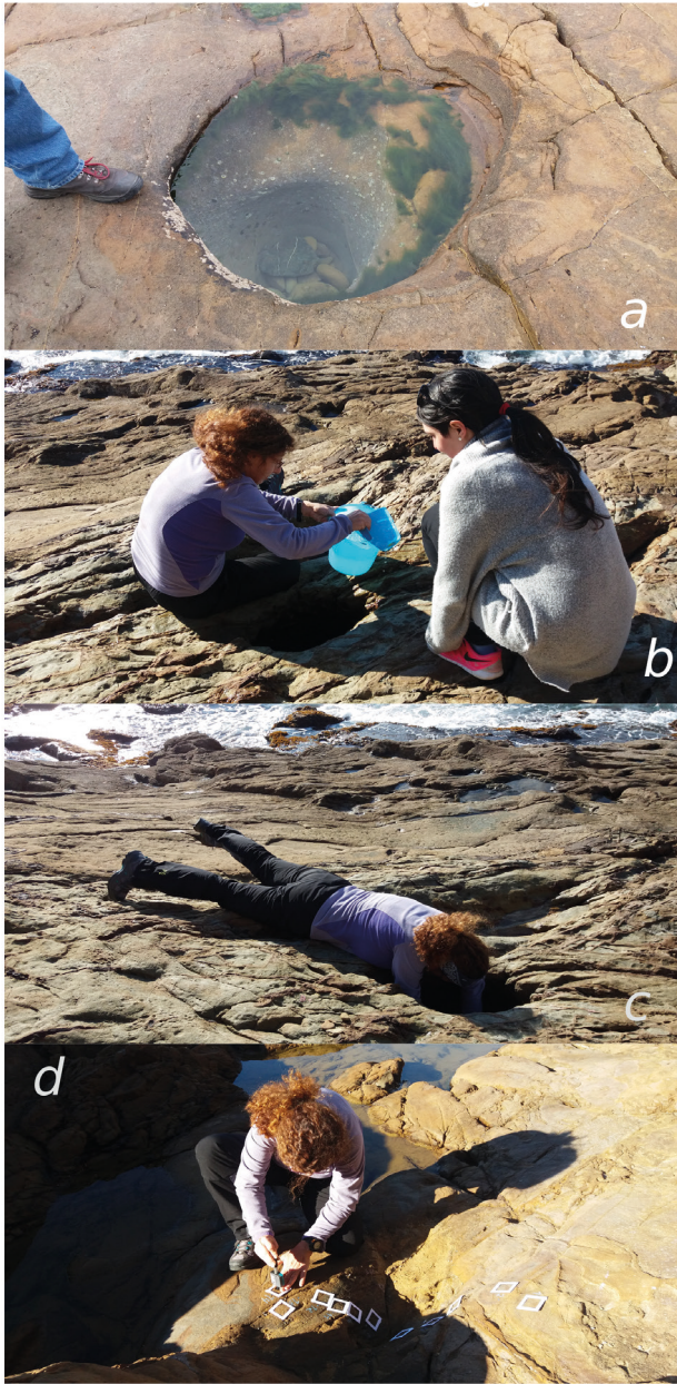
FIG. 3 - The different stages of the experimental protocol: potholes selection (a); extraction of water (b) and of sediments (c); hardness testing (d).
